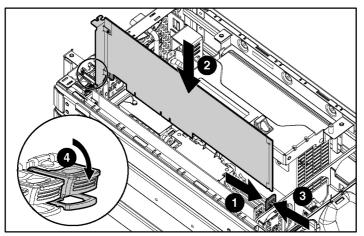
Figure 1-26: Installing an expansion board
